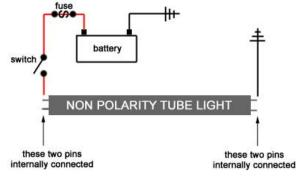
The circuit simplified: One end of the tube light needs a positive power supplied, the other side ground. At each end of the tube, the two pins are interconnected, so you only need a wire connected to one pin at each end (but redundancy is ok)
